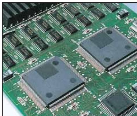
Epoxy-silanes are essential for performance of epoxy resin encapsulants for microchips.
