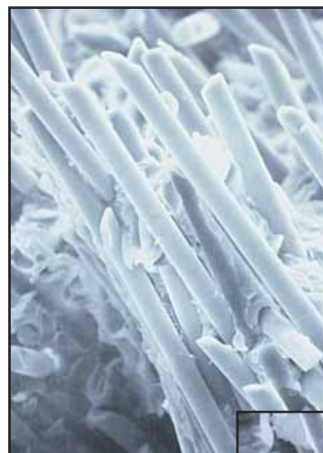
Scanning electron micrograph at a broken gear tooth from an aminosilane-coupled glass fiber/nylon 6/6 composite. Note how fibers have broken as well as matrix.
