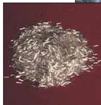
Chopped fiberglass strand sized with aminosilanes is a commonly used reinforcement for high temperature thermoplastics.
